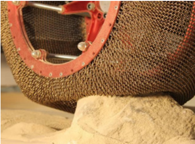
Superelastic tire with shape memory
